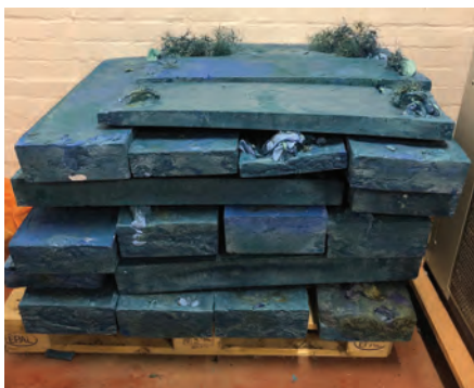
The used surgical wraps are melted down using a process that converts them into a solid polypropylene material.
